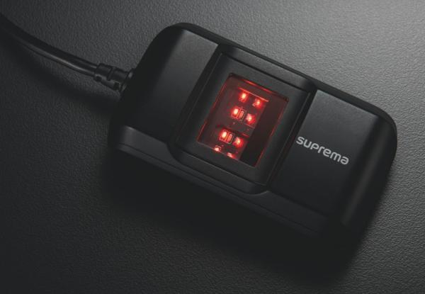
BioMini Slim 2S is a FBI PIV and Mobile ID FAP20 certified fingerprint scanner that provides a number of industry-leading features under its sleek design. Featuring range-leading powerful 1.0GHz CPU, BioMini Slim 2S provides high-speed extraction and matching of fingerprints within the scanner.
